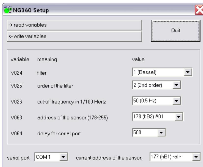
After that, invoking "read variables" returns the desired sensor's current configuration and displays the values in the corresponding boxes.
