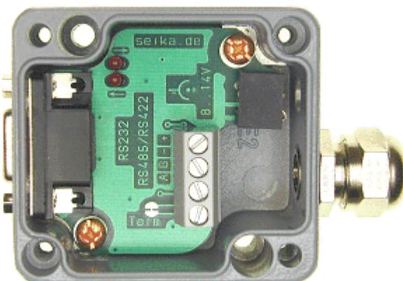
**RS232 / RS485 interface converter for connection of SEIKA sensors with RS485 interface to RS232 port of a computer**
