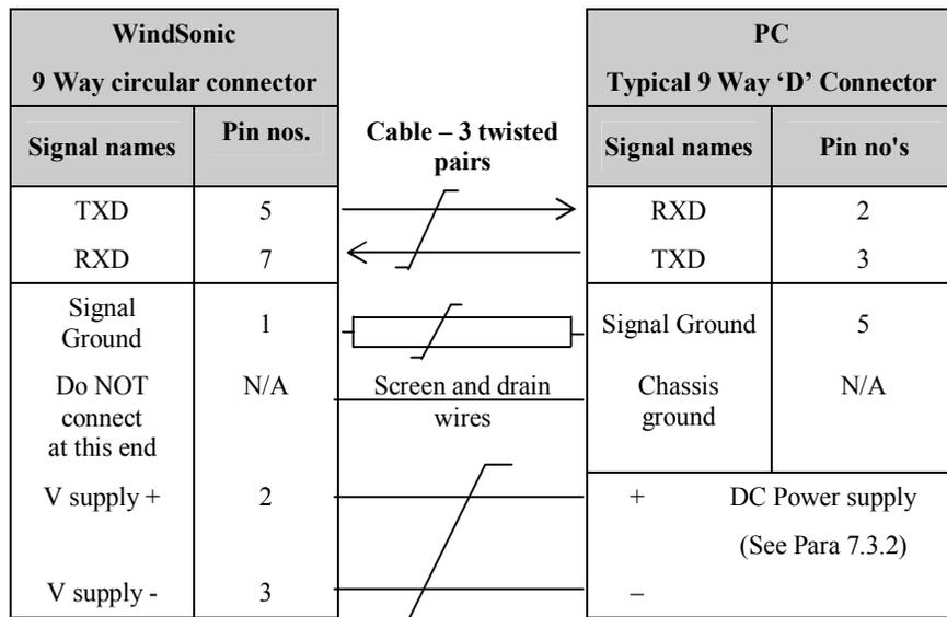
Connect the Option 2 or 3 WindSonic as per the above connection diagram.
