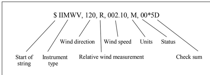
The **Wind Direction**, **Wind Speed**, and **Units** are as described in Section 9.1.
