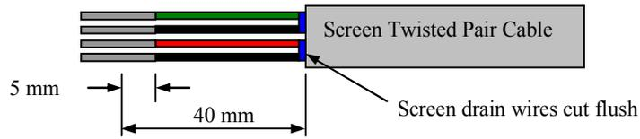
Put the parts on the cable in the order as shown below.
