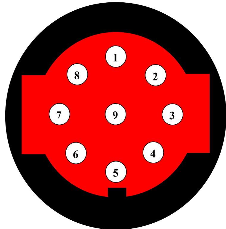
Continue to insert all of the contacts you require. Once all of the contacts are inserted push the red retainer into place. NB. The retainer can only be pushed back into place if the contacts are fully engaged.
