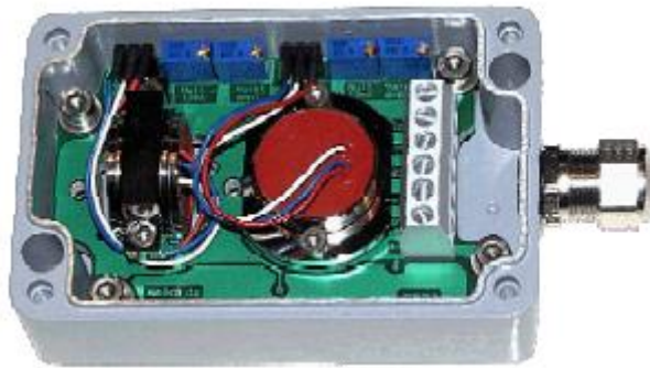
Sensor box containing two sensors and two signal conditioners with 4...20mA, 2-wire outputs
