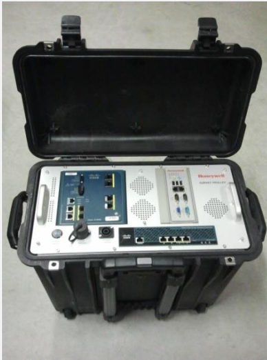
Portable ethernet server for field applications (Running on batteries)
