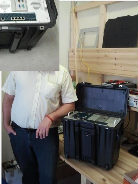
Portable ethernet server for field applications (Running on batteries)
